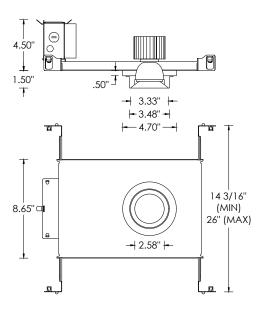
NC - NEW CONSTRUCTION HOUSING (NON-IC AND CP RATED)
