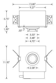
**SH -** SHALLOW HOUSING (IC AND CHICAGO PLENUM RATED) (2200LM MAX)
