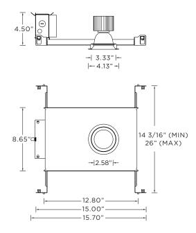
NC - NEW CONSTRUCTION HOUSING (NON-IC AND CP RATED)
