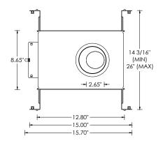
**NC -** NEW CONSTRUCTION HOUSING (NON-IC AND CP RATED) IC - NEW CONSTRUCTION IC HOUSING (2200LM MAX)
