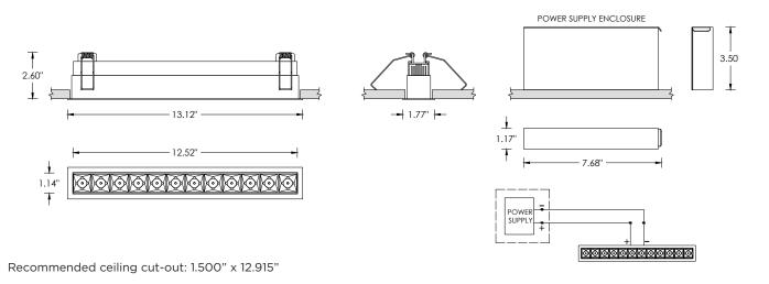
SH - SHALLOW HOUSING (INTEGRAL DRIVER) (IC RATED AND CHICAGO PLENUM RATED)
