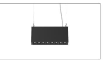
8 Light high performance pendant with 1" apertures Narrow 1.5" aperture with one piece extruded aluminum housing LED system delivers over 1600lm at 90+ CRI Features matte black or matte white multi-faceted louvers Regressed LED source with enhanced glare control, UGR <16 100-1% dimming range standard with integral drivers
