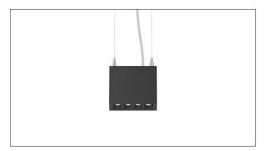
4 Light high performance pendant with 1" apertures Narrow 1.5" aperture with one piece extruded aluminum housing LED system delivers over 800Im at 90+ CRI Features matte black or matte white multi-faceted louvers Regressed LED source with enhanced glare control, UGR <16 100-1% dimming range standard with remote drivers
