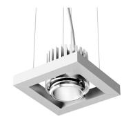
Extruded aluminum frame with fabricated mitered corners Standard clear etched and black etched anodized finishes Machined aluminum double gimbals. Adjustable and lockable Regressed LED source for enhanced glare control Lumen range of 1000lm to 5000lm (80+, 90+, and 97+ CRI options) 1% dimming standard with several integral driver options
