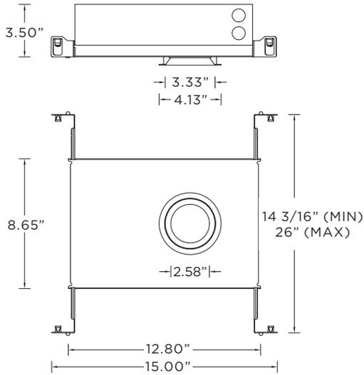
**NC - New Construction Housing (Non-IC) (Chicago Plenum Rated)**
