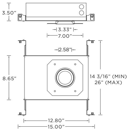
**NC - New Construction Housing (Non-IC) (Chicago Plenum Rated)**
