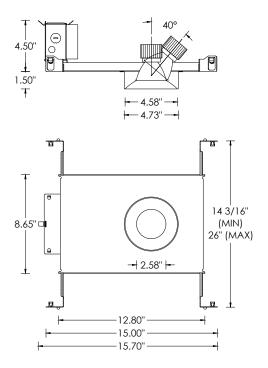
**NC -** NEW CONSTRUCTION HOUSING (NON-IC AND CP RATED) **IC -** NEW CONSTRUCTION IC HOUSING
