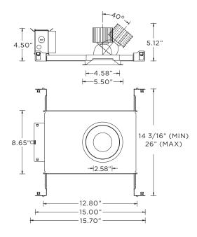
NC - New Construction Housing (Non-IC) (Chicago Plenum Rated)
