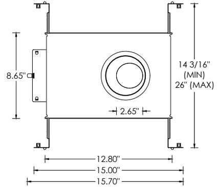
**NC- NEW CONSTRUCTION HOUSING (NON-IC AND CP RATED)**
