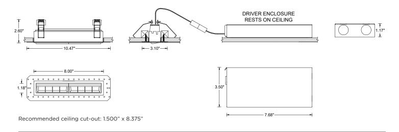
**SH -** SHALLOW HOUSING (INTEGRAL DRIVER) (IC RATED AND CP RATED)
