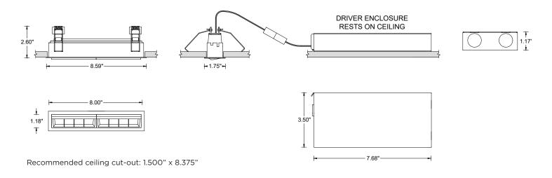
SH - SHALLOW HOUSING (INTEGRAL DRIVER) (IC RATED AND CP RATED)
