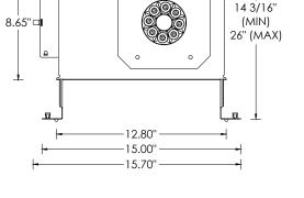
NC- NEW CONSTRUCTION HOUSING (NON-IC AND CP RATED)
