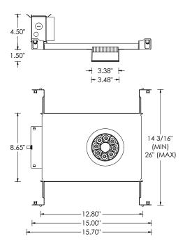
**NC-** NEW CONSTRUCTION HOUSING (NON-IC AND CP RATED) **IC -** NEW CONSTRUCTION IC HOUSING (2000LM MAX)
