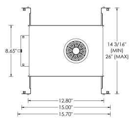
NC- NEW CONSTRUCTION HOUSING (NON-IC AND CP RATED)
