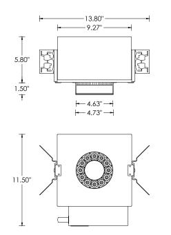
SH- SHALLOW HOUSING (IC AND CP RATED) (2500LM MAX)(SHIPS WITH BAR HANGERS)
