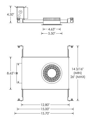
NC- NEW CONSTRUCTION HOUSING (NON-IC AND CP RATED) IC - NEW CONSTRUCTION IC HOUSING (2500LM MAX)
