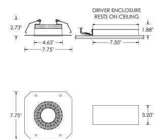
SH- SHALLOW HOUSING (IC AND CP RATED) (2500LM MAX)(SHIPS WITH BAR HANGERS)
