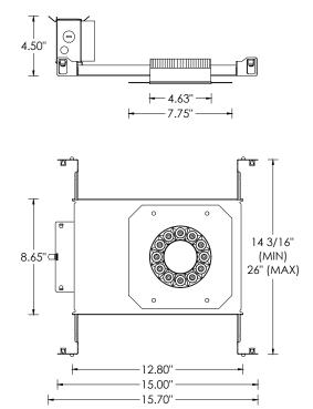
NC- NEW CONSTRUCTION HOUSING (NON-IC AND CP RATED) IC - NEW CONSTRUCTION IC HOUSING (2500LM MAX)
