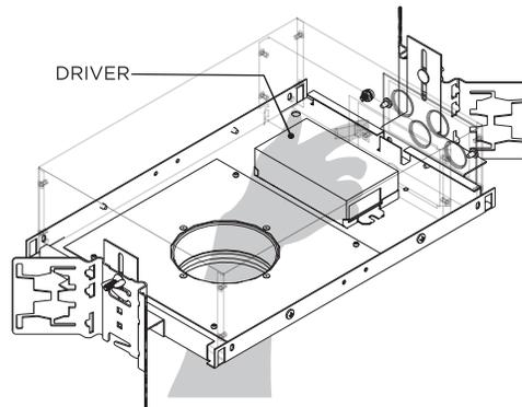
REMOVE DRIVER - SECURED WITH HOOK-AND-LOOP FASTENER
