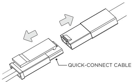
DISCONNECT QUICK-CONNECT CABLE FROM LED ASSEMBLY
