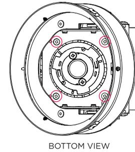
LOCATE AND REMOVE THE FOUR HIGHLIGHTED SCREWS
