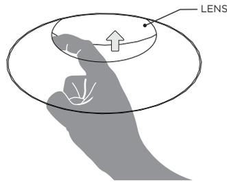
LIFT LENS AND DETACH INSERT FROM ADAPTER RING
