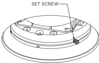
LOOSEN THREE SET SCREWS INSIDE ADAPTER RING
