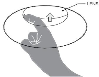
LIFT LENS AND DETACH INSERT FROM ADAPTER RING
