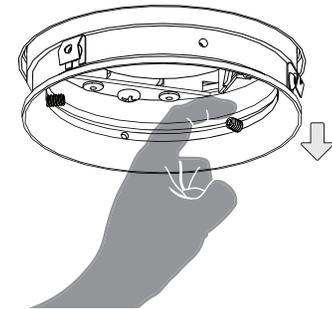
UNCLIP ADAPTER RING FROM CEILING BY PULLING DOWN ON EACH SET SCREW
