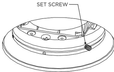
LOOSEN THREE SET SCREWS INSIDE ADAPTER RING
