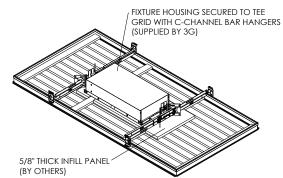
**PLEASE NOTE:** FIXTURE INSTALLATION MUST BE COORDINATED WITH CEILING PANEL INSTALLATION TO ENSURE FIXTURE ACCESSIBILITY CEILING SYSTEM AND 5/8" THICK INFILL PANEL (BY OTHERS)
