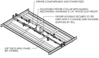
PLEASE NOTE: FIXTURE INSTALLATION MUST BE COORDINATED WITH CEILING PANEL INSTALLATION TO ENSURE FIXTURE ACCESSIBILITY CEILING SYSTEM AND 5/8" THICK INFILL PANEL (BY OTHERS)
