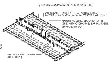
**PLEASE NOTE:** FIXTURE INSTALLATION MUST BE COORDINATED WITH CEILING PANEL INSTALLATION TO ENSURE FIXTURE ACCESSIBILITY CEILING SYSTEM AND 5/8" THICK INFILL PANEL (BY OTHERS)
