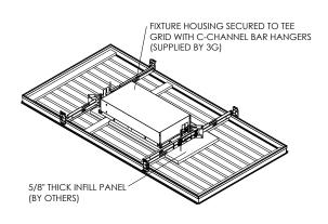
PLEASE NOTE: FIXTURE INSTALLATION MUST BE COORDINATED WITH CEILING PANEL INSTALLATION TO ENSURE FIXTURE ACCESSIBILITY CEILING SYSTEM AND 5/8" THICK INFILL PANEL (BY OTHERS)
